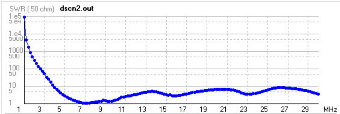
Fig. 10.5A.3 Frequency response of standing wave ratio of a discone antenna (radius of cone d = 4.2 m, the length l = 16.8 m)
