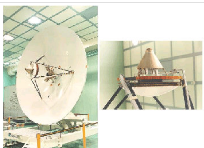
Fig. 6.2 Antenna for the satellite Cassini 96 (left). A detailed view on hyperbolic sub-reflector of this antenna (right).
