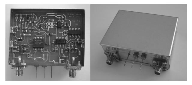
Fig. 2. Realized 5 MHz secondary frequency standard
