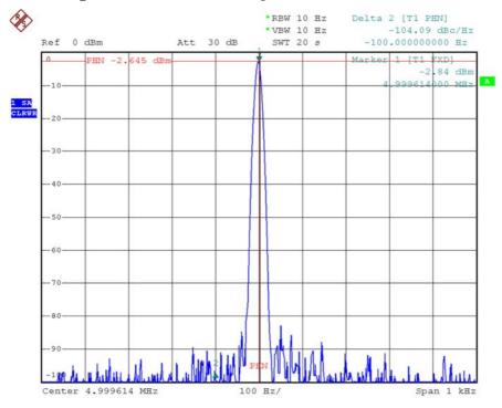
**Fig. 4.** Phase noise of secondary frequency standard output signal in phase lock state
