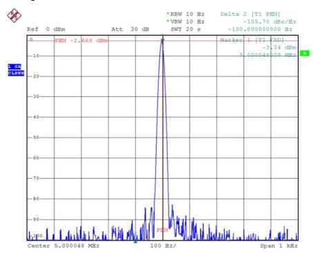
**Fig. 3.** Phase noise of the non synchronized output signal (free running state)
